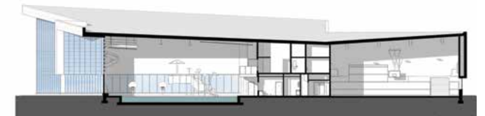
Section 3: East-West through natatorium
