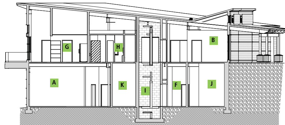
Building section - Vestibule and balcony
