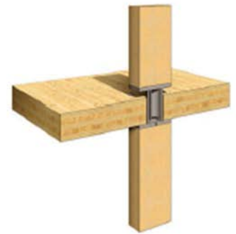
CLT floor slabs with glulam columns and steel connectors
