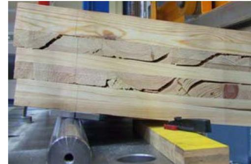
The shear strength for rolling shear is approximately equal to twice the tension strength perpendicular to the grain (EN 1995)
