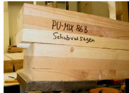
Shear failure in longitudinal layers
