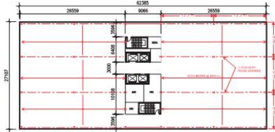
2a. Steel Truss Girders
