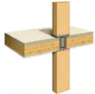
partial encapsulation during construction
