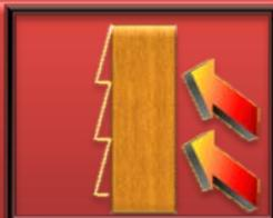
Exterior walls are to be rated for exposure from the inside.
