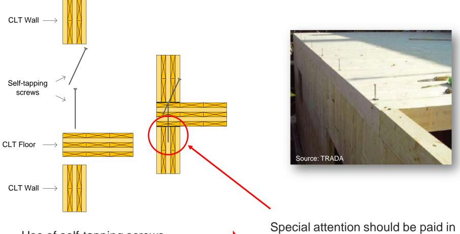
Use of self-tapping screws (Simplest form of connection)
