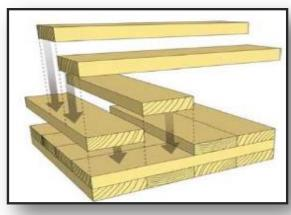
However, <u>need to take into account</u> some of the specific features of panels at the design stage (e.g., gaps, lamination orientation, etc.)
