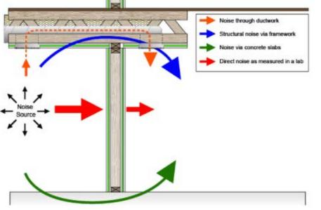
The STC rating corresponds to the dB absorbed by the wall. This wall is rated at STC = 55, so a sound of 80 dB should be heard at 25 dB on the other side of the wall.
