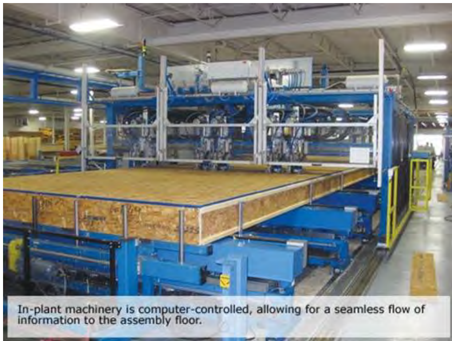
Floor and wall panels are fabricated and assembled ensuring the final product meets the highest standards.
