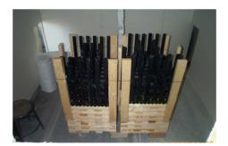
Figure 4. Mixed fuel package of wood cribs and plastic pipes.
