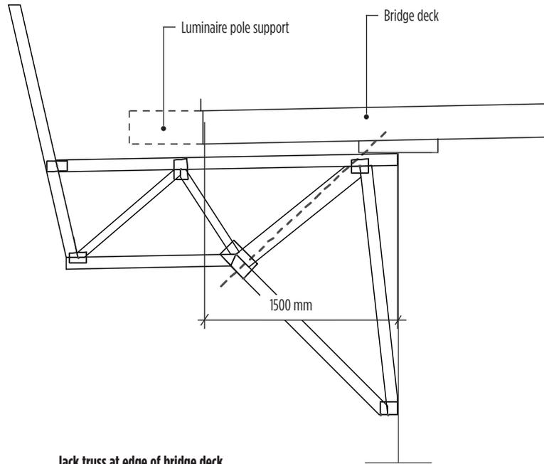
**Jack truss at edge of bridge deck**
