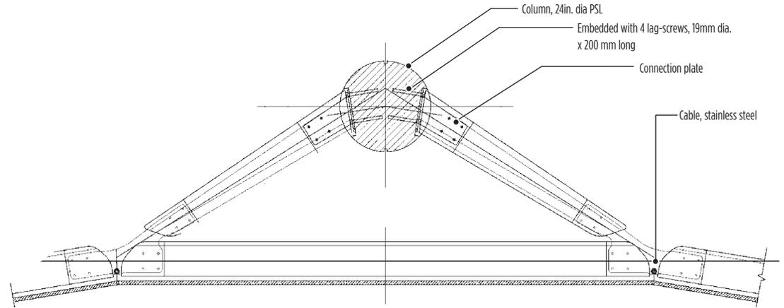
Plan, bracing from column to glazing at facade
