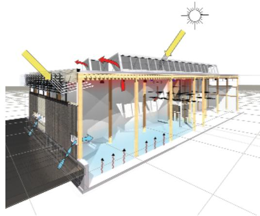
Building section at research wing showing ventilation and radiant floor heating flows
