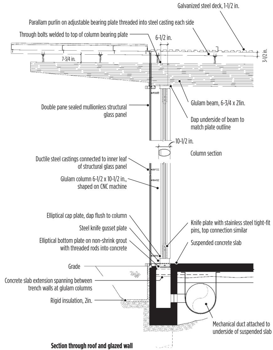
**Section through roof and glazed wall**
