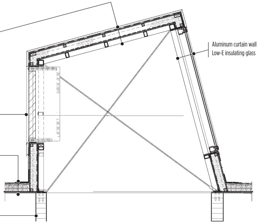
Section through research wing roof monitor
