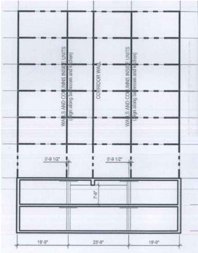
Underground parking becomes more expensive because of the transfer slab required to transfer the loads from the bearing walls to the columns.
