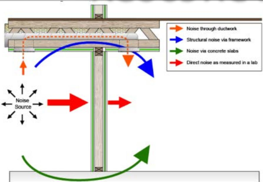
The STC rating corresponds to the dB absorbed by the wall. This wall is rated at  $STC = 55$ , so a sound of 80 dB should be heard at 25 dB on the other side of the wall.
