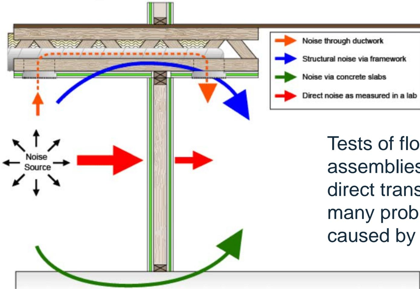
Tests of floor and wall assemblies evaluate direct transmission, but many problems are caused by flanking.
